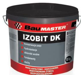
Bituminous mass used in the maintenance of roofing felt, in the execution of jointless waterproofing coatings, laminates reinforced with glass veil, in the execution of top waterproofing of underground parts of buildings and industrial water tanks.
